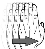
To switch on the extractor hood, move your hand horizontally from left to right about 3-5 cm below the sensor. In this way, the power level changes to a higher gear (2).
