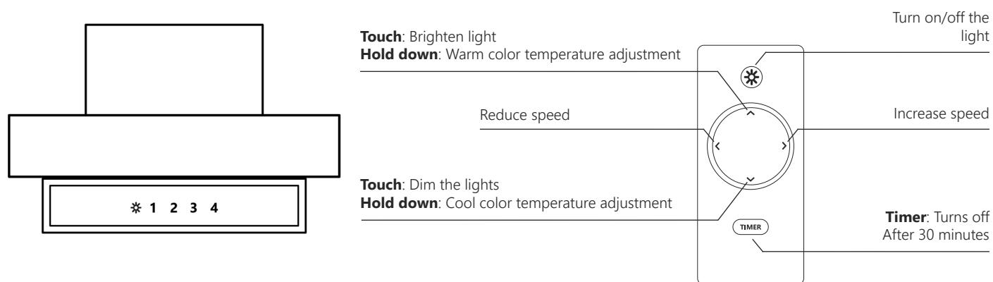
**1 2 3 4 Start/stop the device and adjust the speed from the switch panel tab:** 1, 2, 3, or 4. Speed four is an intensive power that always returns to speed three after 5 minutes. The device can also be turned off/started by turning the lid open or closed under the device.
